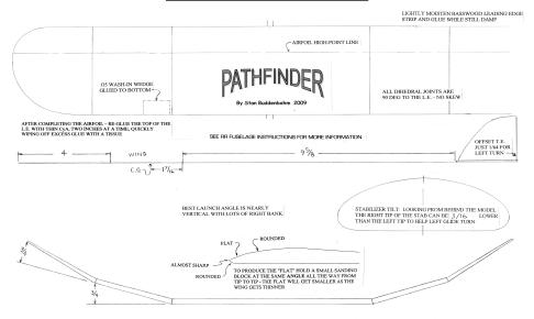
PATHFINDER 16" span 5 panel wing with a 3" chord. Simple outlines, easy construction. The straight airfoil high point line makes for easier shaping. **Many Wins** including the 2009 Nationals. Great launch height. Includes RR fuselage with built in viscous timer.
