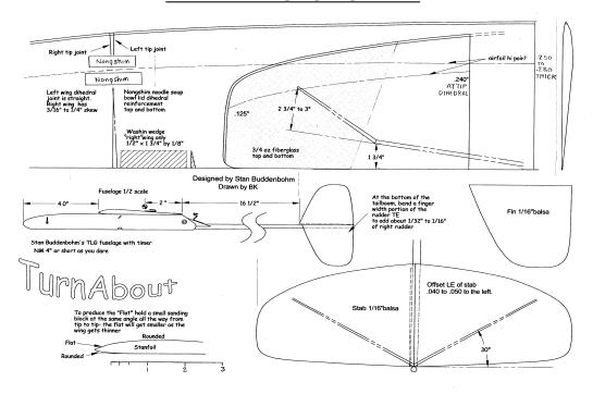
TURNABOUT is a 36" span (before dihedral) TLG. The design features a change in the dihedral scheme which provides a very forgiving transition from launch to glide. TurnAbout has already won some contests as well as third at the 2018 Nationals. Kit includes the pop up tail boom fuselage with viscous timer built in. My current favorite.
