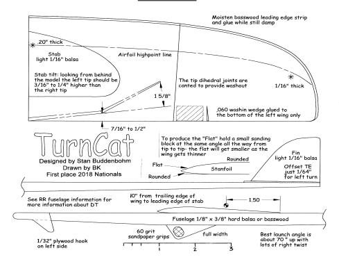
TURNCAT is a 16" span design that has won the 2018 Nationals and the 2019 Southwest Regionals at Eloy, AZ. Tremendous launch height with a beautiful transition to glide. Easy to shape wing. Can be ordered with a simple wooden fuselage and no DT, or with the RR pop up wing that has my viscous timer built in.
