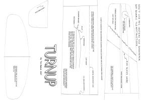
TURNUP designed by Tim Batiuk 36" span, 4.5 inch chord. Many wins and holder of the current National record with 23 MAXES. Need I say more? Kit includes pop up tail boom fuselage with my built in viscous timer.
